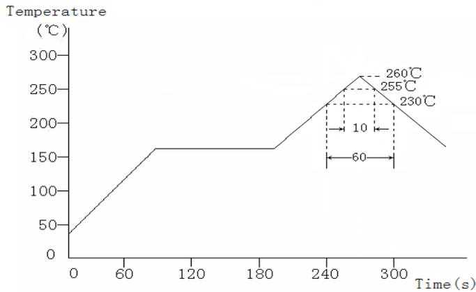
No mechanical and electrical defects are found after testing based on the above profile and keeping under the conditions of room temperature and humidity for 2 hours.
