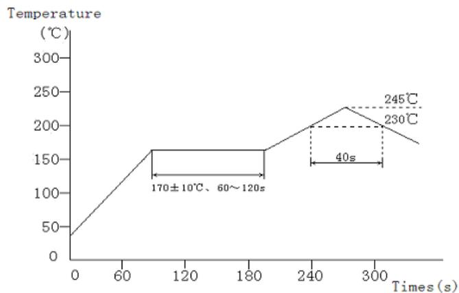
The recommended reflow profile is based on the testing instruments used. Solder ability will reflow conditions, testing method, etc. So it is necessary to make a confirmation of them when the reflow conditions are set up.
