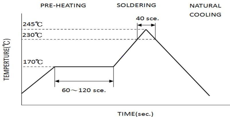
The recommended reflow profile is based on the testing instruments used. Solder ability will depend on the testing equipments, reflow conditions, testing method, etc. So it is necessary to make a confirmation of them when the reflow conditions are set up.
